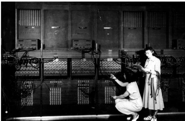
*A small amount of time is required in preparing the ENIAC for a problem by such steps as setting program switches, putting numbers into the function table memory by setting its switches, and establishing connections between units of the ENIAC for the communication of programming and numerical information. (Pressemitteilung, DoD, 1946)*
